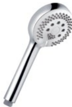
KLUDI-LOGO | hand shower 3S DN 15 booster, smooth, volume flow rate 9 l/min at 3 bar
