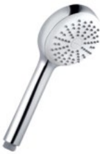
KLUDI-LOGO | hand shower 1S DN 15, volume flow rate 41 l/min at 3 bar
