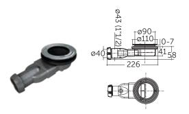
**KLUDI-TERRA** Shower Drain membrane water seal discharge rate 0.5L/s
