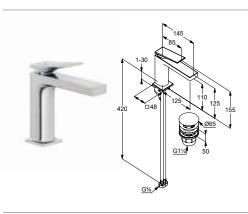
KLUDI-DECUS single lever basin mixer 110 DN 15 single hole mounted solid lever s-pointer-aerator M 18,5 x 1 ceramic cartridge with hot water limitation flow rate 5 l/min. at 3 bar flexible pressure hoses G 3/8 DVGW approved rapid installation set PUSH-OPEN waste G 1 1/4
