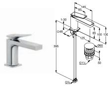
**KLUDI-DECUS** single lever basin mixer 85 DN 15 single hole mounted solid lever s-pointer-aerator M 18,5 x 1 ceramic cartridge with hot water limitation EcoPlus centre position cold water flow rate 5 l/min. at 3 bar flexible pressure hoses G 3/8 DVGW approved rapid installation set PUSH-OPEN waste G 1 1/4
