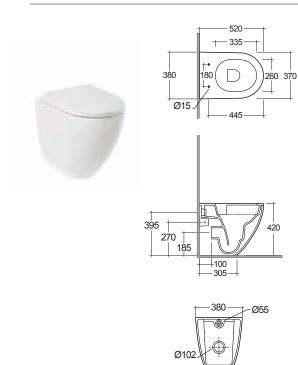
**Product description** Surface KLUDI-RESA D Glossy White Floor-standing toilet Dimensions (cm): W: 37 H: 42 D: 52 Spiralflush technology Universal-shaped outlet Flushing performance 3/6l Full flush toilet Concealed Fischer fixation EN 997 - CL1 - 6A
