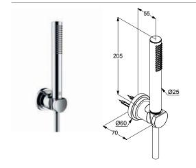
Classic bath shower set 1S hand shower DN 15 with spray mode: volume flow rate 11 l/min at 3 bar quick and easy cleaning system KLUDI-SUPARAFLEX hose anti twist G 1/2 x G 1/2 x 1250 mm plastic-coated with conical nuts fixed wall shower hook with screws and dowels wall fastening Chrome
